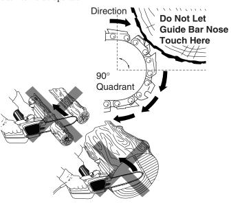
Figure 1 - Kickback Hazard Example. Do Not Let Nose of Guide Bar Touch Object While Chain is Moving
